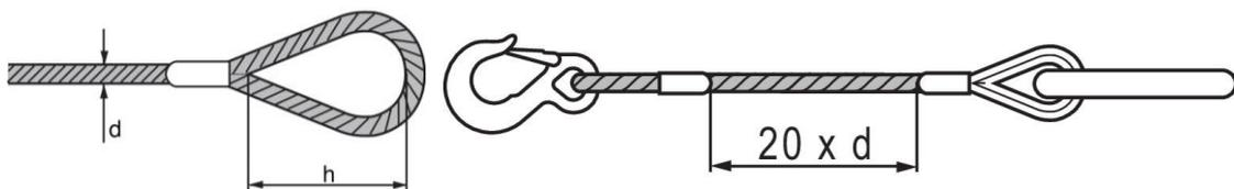
The minimum length of straight rope between the inside ends of ferrules terminating a sling eye shall be 20 times the nominal rope diameter.
