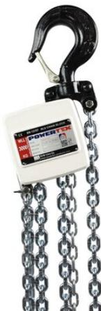
Extremely small and lightweight aluminum chain block. It weighs only approximately 50% of a similar standard chain block. The block can be used for lifting as well as pulling. The hoists are factory equipped with overload protection device (OLP), which limits the maximum operating force that can be applied using the hand chain.
